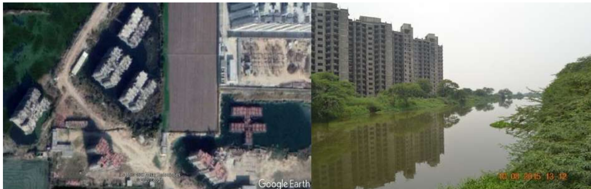
Picture 5. Wetland areas wherever constructed upon are routinely under water. Left: Apartment in Sector 107 inundated; Right: Woodshire Apartments of Sector 108 Gurgaon having with basement and lower storeys inundated)
